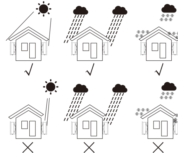
Figure 5.1 Recommended Installation locations
